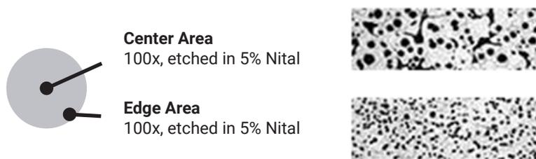
The microstructure consists of Types I & II nodular graphite as defined in ASTM A247. The matrix is ferrite with approximately 5-25% pearlite. The edge or rim will have a higher nodular count and will be mostly ferrite. Chill carbides will be less than 5% in any field at 100x and will be well dispersed.
