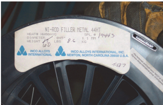
Label on a Spool of Special Metals NiRod Filler for Welding Iron
