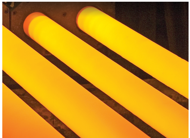
The resulting bar stock is free of dross, slag, sand, virtually all porosity and other impurities that create machining problems, which increase the cost of finished goods.
